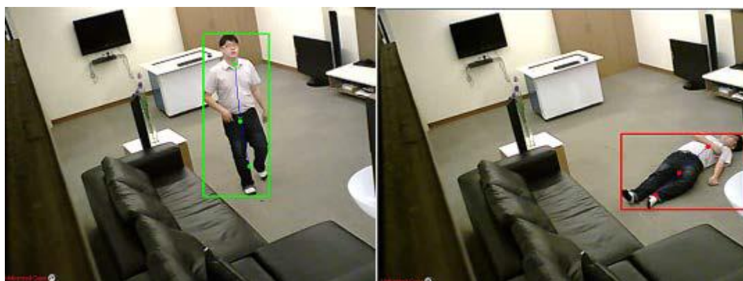
Figure 15: Visual examples of a normal detection (green blob on the left) and a fall detection (red blob on the right).
